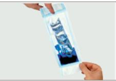
Wait for 20 second, no longer, (if testing all 4 seals, allow 5 seconds ink contact on each)
